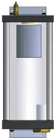
P7306 - 1 Gallon Pressure Pot A one gallon Pressure Pot to feed fluid under pressure. Clear reservoir, pressure regulator for air in and a solenoid valve at the fluid out port. Includes a 30PSI pop-off valve.
